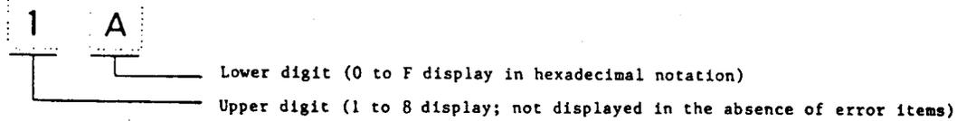
2. For error codes, error conditions for four items in the lower digit and three items in the upper digit are displayed in a hexadecimal notation code.
