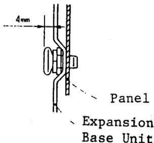
Applicable screw: M4 pan-head screw (spring or flat washers may be used.) (These are not attached to the unit.)
