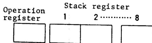
The stack register is so designed that the execution of one LOD instruction shifts down the stored results by one stack register, and the execution of one AND LOD or OR LOD instruction as explained later shifts them up by one stack register. The operation results can be stored in this stack register eight times continuously.
