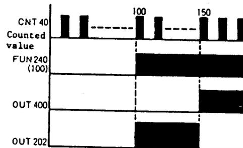
Output 202 is turned ON when Counter 40 counted value is between 100 and 150.
