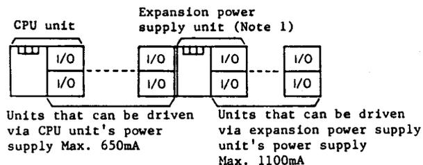
Note 1: Two input or output units can be loaded on expansion power supply unit.
