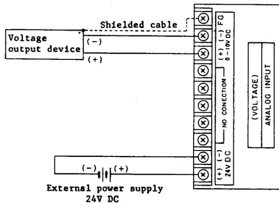
**Note: NO CONNECTION Terminals - Do not connect input and other wiring.**
