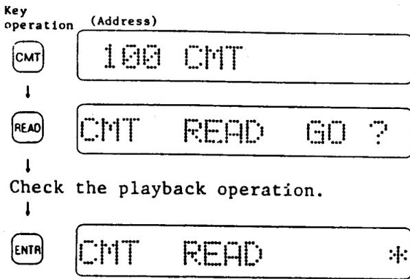
Simultaneously with pressing the ENTR key, set the cassette tape recorder to the PLAY mode.
