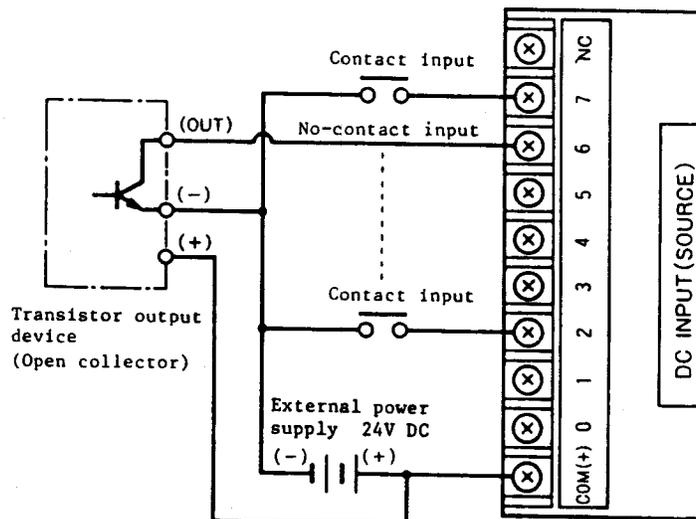
Note: NC (No Connection) - Do not connect input and other wiring.
