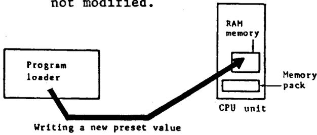
The RAM memory (new preset values for timer and counter) in the CPU unit is preserved for about one week (at 25°C) after power failure. However, when a CMOS-RAM pack is used, the memory is backed up by a battery in the memory pack.
