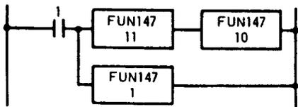
When input is turned ON, 8-bit BCD data of input Nos. 10 to 17 are read, converted into BIN (binary) values and set at DR0.
