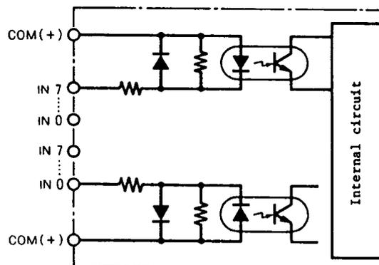
Note: External power supply is required for input.
