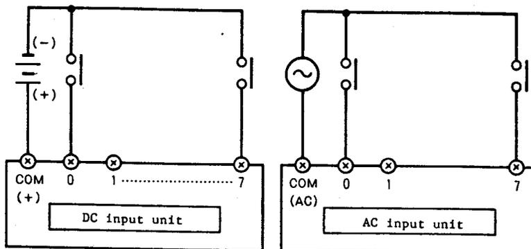
Note: Be sure to avoid contact between COM (+), COM (-) and COM (AC) of input units.
