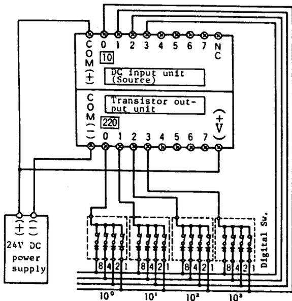
Note 3: Initial input and output numbers are allocated via FUN30 and 31.
