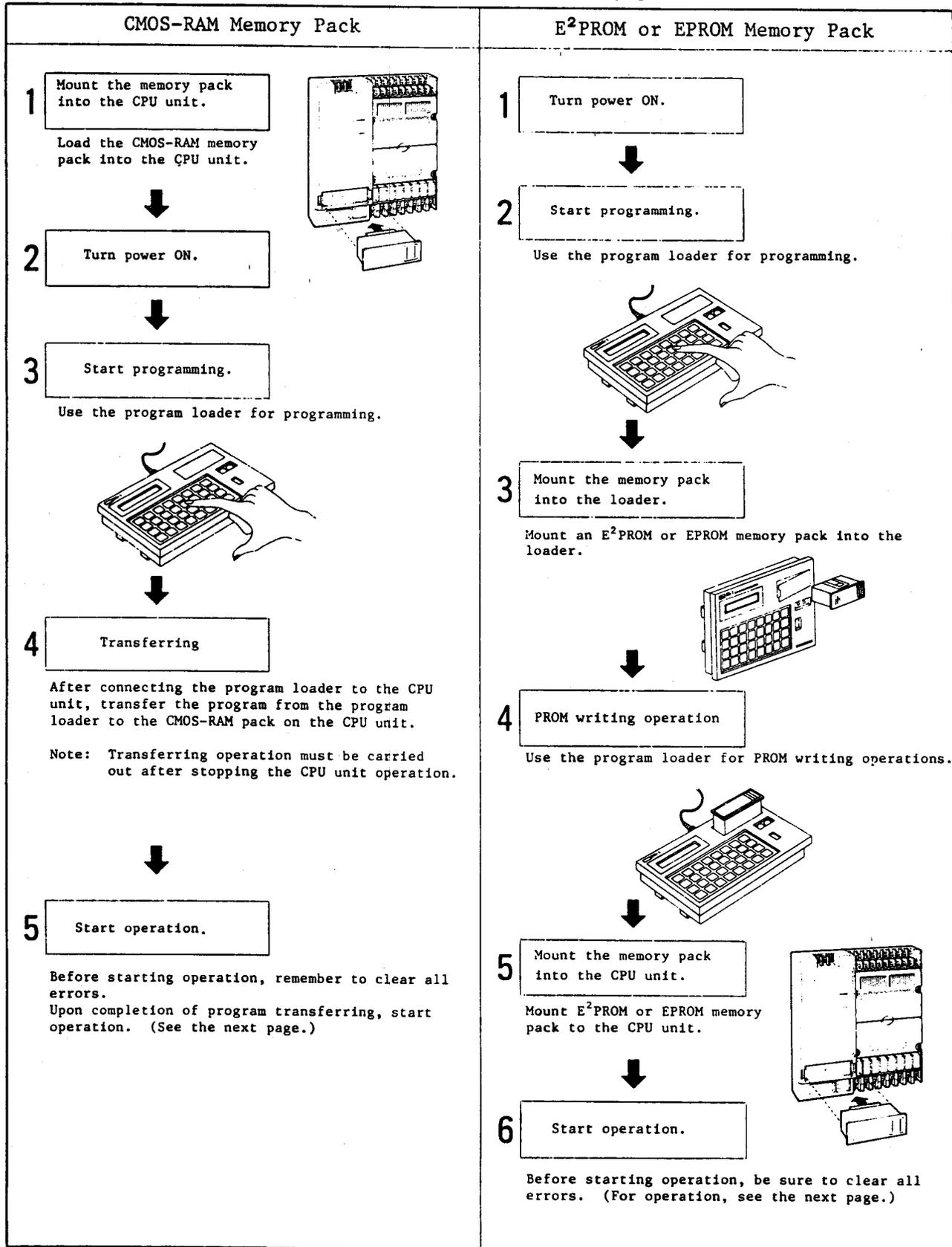
Note: In a system using an E<sup>2</sup>PROM, use a RAM memory pack when the system is started up: this can reduce the time required for transferring the program.
