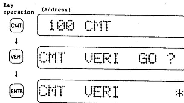
Simultaneously with pressing the ENTR key, set the cassette tape recorder to the PLAY mode.
