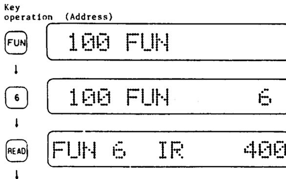
To designate clear type internal relays Nos. 500 to 697: (Nos. 400 to 497 are designated as keep type internal relays.)
