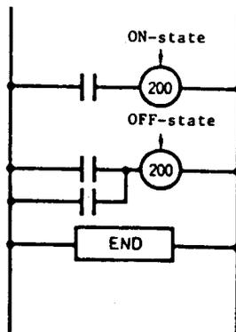
In this example, output 200 is OFF. Under this condition, if output 200 is monitored, it is blinking at random.
