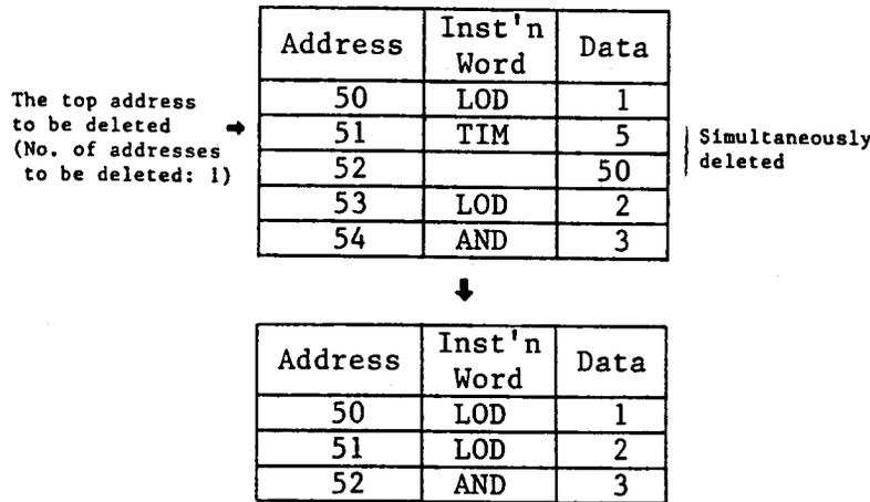
The top address to be deleted (No. of addresses to be deleted: 1)
