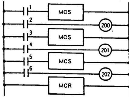
The above master control circuit gives priority to Input 1, Input 3, and Input 5 in this order.
