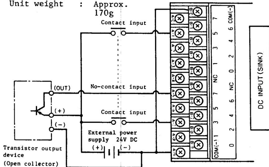
Note 1: NC (No Connection) - Do not connect input and other wiring.
