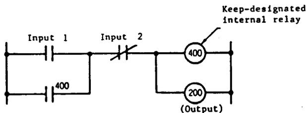
[Ex. 2] When a keep type internal relay is self-maintained by the SET instruction, the status before power failure is also stored in the memory.
