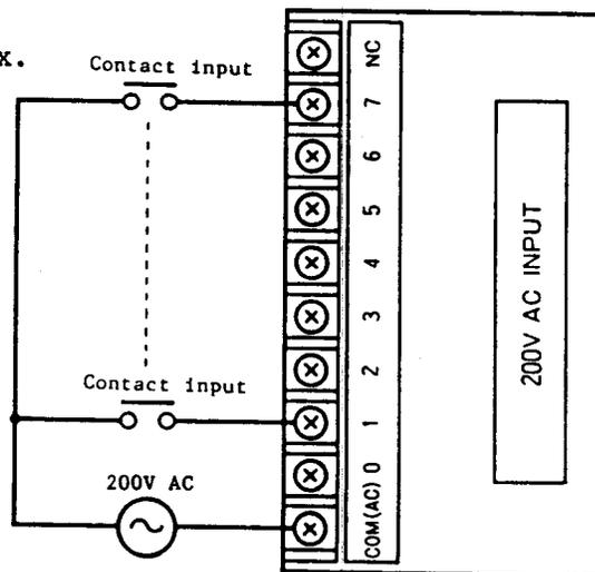
Note: NC (No Connection) - Do not connect input and other wiring.
