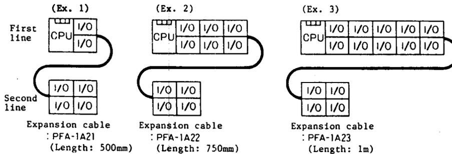
Note: Fix the I/O expansion cable on a mounting plate; instead of installing it in a wiring conduit.
