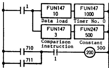
Note: Be sure to program an AND circuit with the contact for execution and comparison result 710, 711 and 712 contacts.
