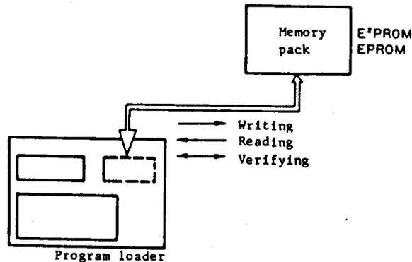
Note: Do not write, readout or verify a CMOS-RAM memory pack. The program may be possibly changed.
