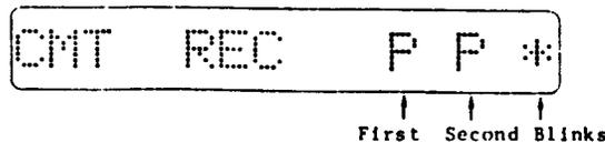
When recording is completed three times, the following message is displayed.
