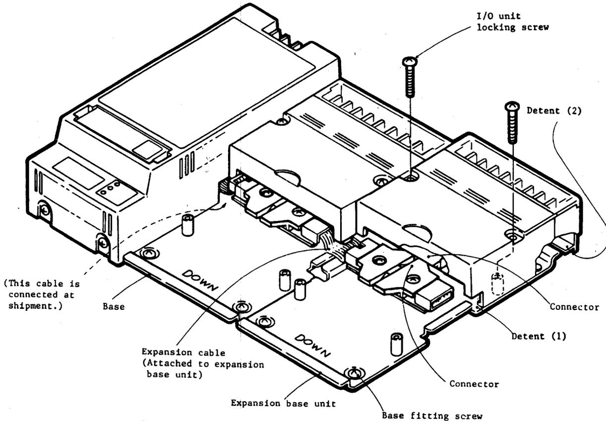
Connection of expansion cable PFA-1A21/PFA-1A22/PFA-1A23 to expansion power supply unit's expansion connector IN side
