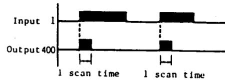
Note 1: If operation is started with input signal ON, the SOT output does not turn ON. To turn on the SOT output, input signal must turn on after starting operation.
