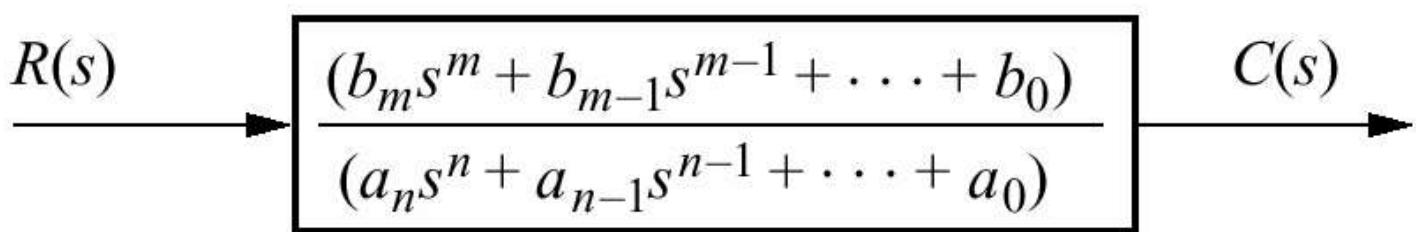
$$\frac{C(s)}{R(s)} = G(s) = \frac{(b_m s^m + b_{m-1} s^{m-1} + \dots + b_0)}{(a_n s^n + a_{n-1} s^{n-1} + \dots + a_0)}$$
