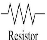
$$v(t) = Ri(t) \quad i(t) = \frac{1}{R} v(t) \quad v(t) = R \frac{dq(t)}{dt} \quad R \quad \frac{1}{R} = G$$
