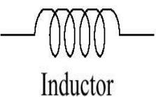
$$v(t) = L \frac{di(t)}{dt} \quad i(t) = \frac{1}{L} \int_0^t v(\tau) d\tau \quad v(t) = L \frac{d^2q(t)}{dt^2} \quad L_s \quad \frac{1}{L_s}$$
