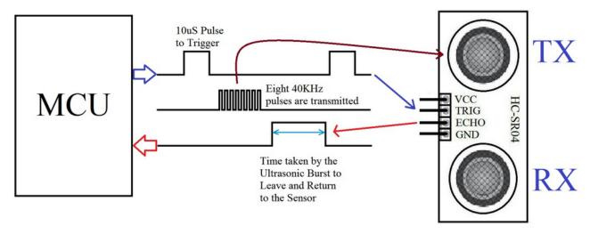
Figure-5: Microcontroller Interfacing
