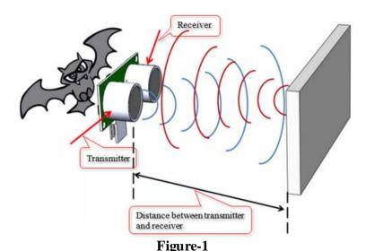
HC-SR04 Ultrasonic Sensor is a very affordable proximity/distance sensor that has been used mainly for object avoidance in various robotics projects. It has also been used in turret applications, water level sensing, and even as a parking sensor.
