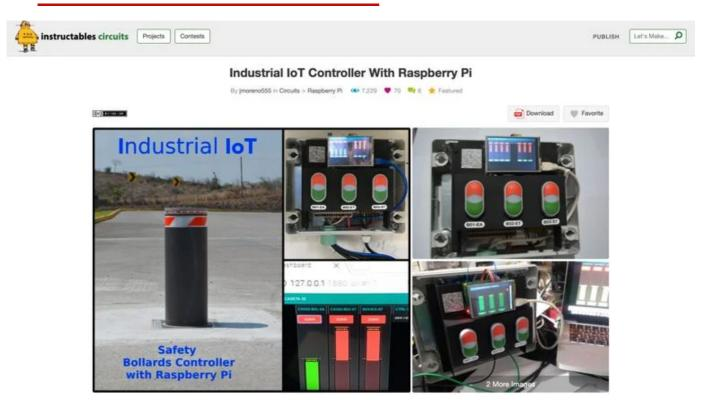
The Raspberry Pi has proven an excellent alternative to programmable logic controllers, a standard in many industries including automation and manufacturing. It is relatively inexpensive and efficient at carrying out programmed tasks through its GPIO interface. Its makers have even designed a board dedicated for its implementations in industrial settings: the Raspberry Pi Compute Module.
