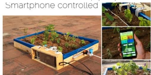
A smart garden checks on the plants' environment to ensure the optimal conditions for them to grow. This project automatically waters plants when the soil is dry. It even turns on the lights when it gets too dark.
