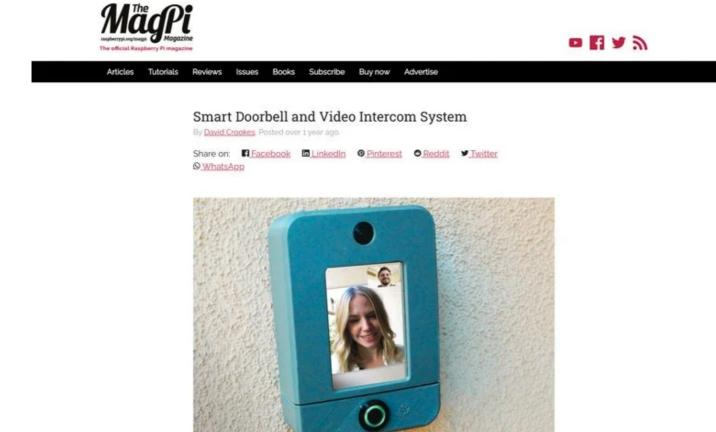
At the heart of this DIY smart doorbell is a Raspberry Pi 3B connected to an LCD display, a camera, STEMMA speaker, and a plug-and-play amplifier.
