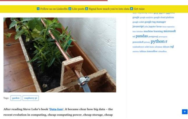
As its name suggests, this is a mini garden that you can water from anywhere in the world! The hardware for this project includes a Raspberry Pi 3B, jumper wires, relay, water pump,
