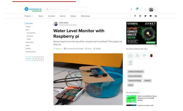
Water level monitoring is used in water treatment applications, such as for pump control and channel flow measurements. Although this simple system works with a bucket of water, it demonstrates this principle, and was was made with a Raspberry Pi 3 Model B, an ultrasonic distance sensor, buzzer, and some jumper wires.
